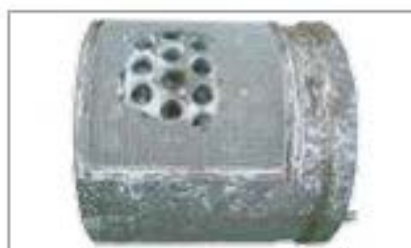
Strainer Screen Damage
