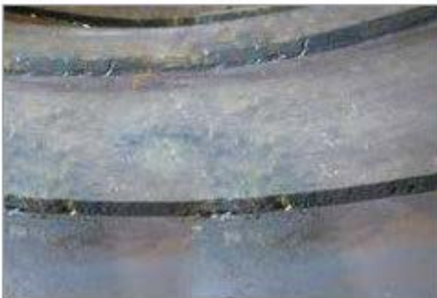
BFPT Casing Seal Face Damage
